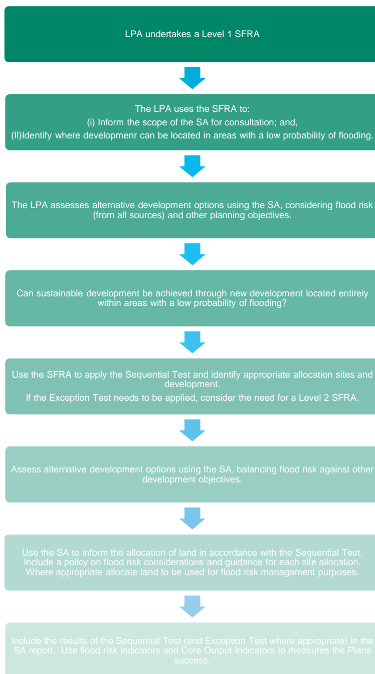
Figure 2.1 Taking flood risk into account in the preparation of a Local Plan (PPG Flood Risk and Coastal Change, p6)
