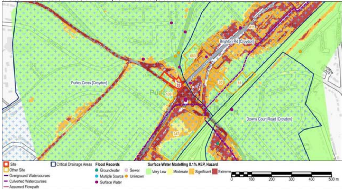
Figure 10 - Surface Water Modelling 0.1% AEP Flood Hazard
