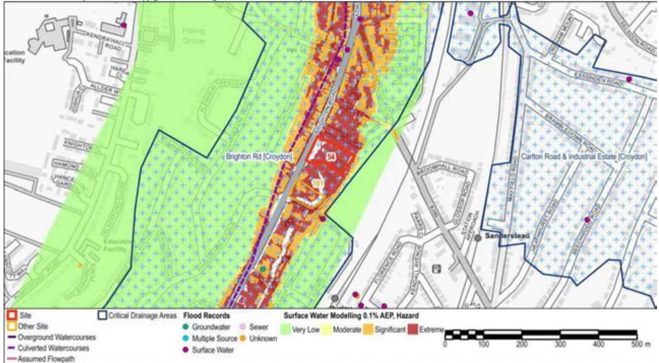
Figure 10 - Surface Water Modelling 0.1% AEP Flood Hazard
