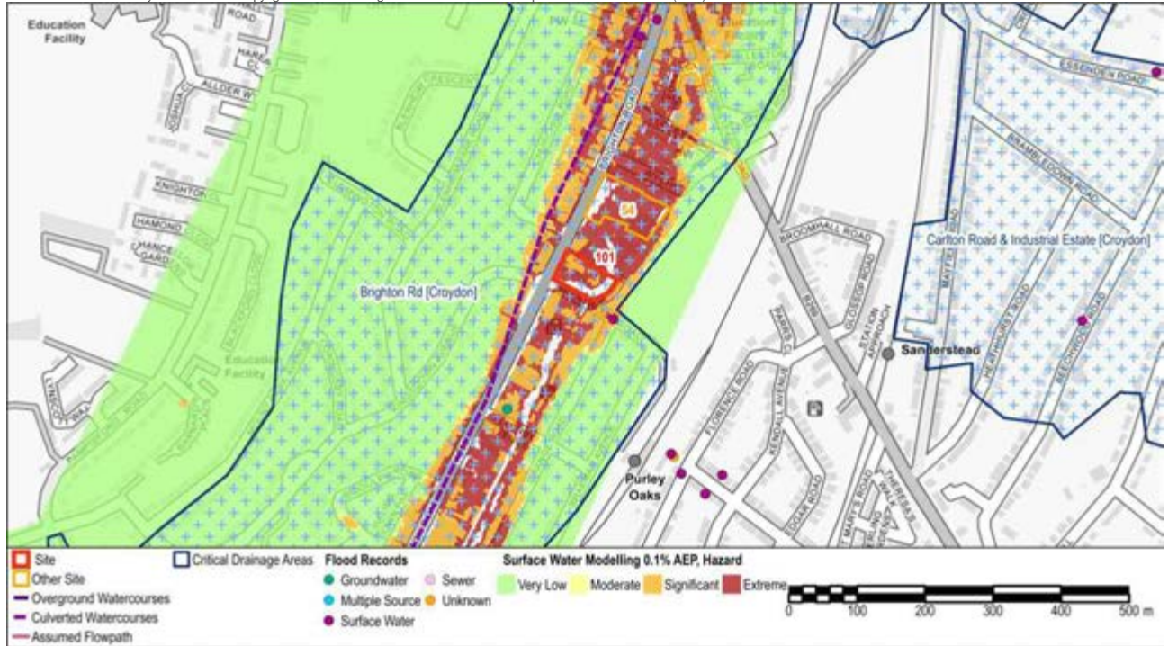
Figure 10 - Surface Water Modelling 0.1% AEP Flood Hazard
