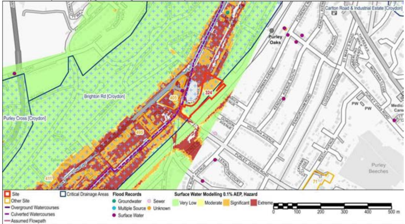
Figure 10 - Surface Water Modelling 0.1% AEP Flood Hazard
