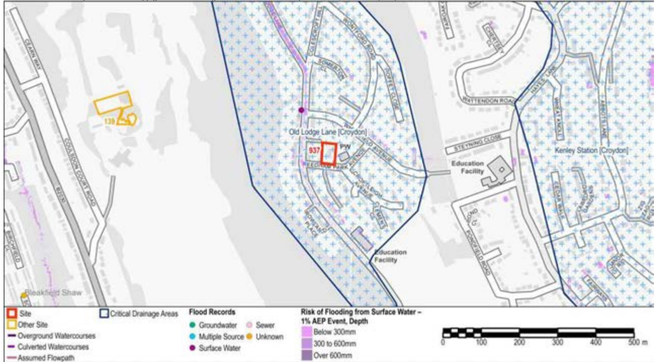
Figure 5 - Risk of Flooding from Surface Water (RoFSW) 1% AEP Flood Depth
