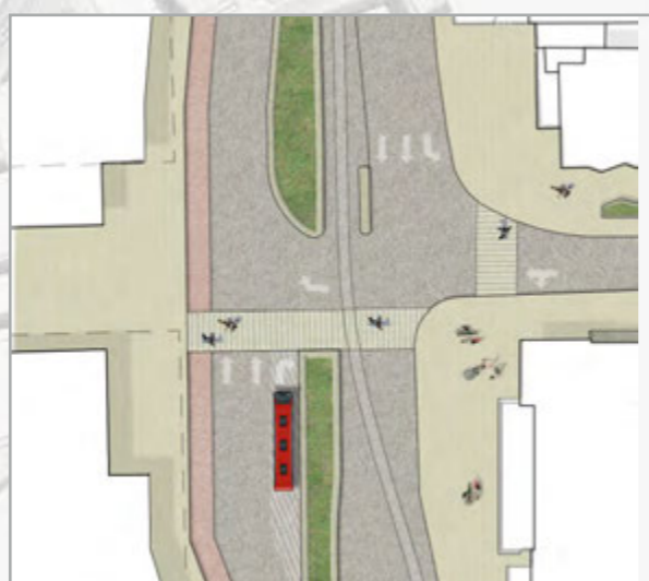
Upgrades required at Wellseley Road/Lansdowne Road Junction (subject to further feasibility testing)
