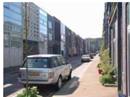
New residential development should provide a continuous building line with frequent entrances and windows. This allows for increased opportunities for surveillance and activity.
