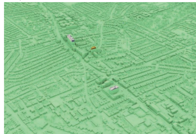
Fig 141 View demonstrating the upper threshold with green datum line set at approximately 33m, equivalent to 10 storeys
