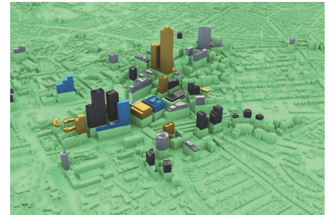
Fig 118 View of the East Croydon station area demonstrating the outer zone minimum threshold with green datum line set at approximately 33m (equivalent to 10 storeys)
