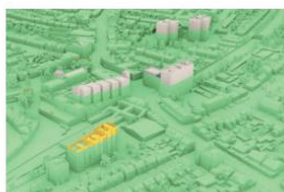
Fig 227 View demonstrating the minimum threshold with green datum line set at approximately 21m (equivalent to 6 storeys)
