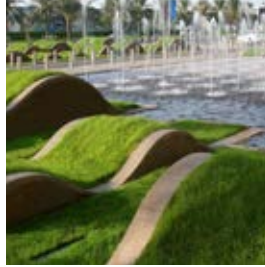
Example of topographical changes integrated in the landscape to create an HVM barrier
