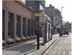
Bus stop backing onto the carriageway to make the most of a narrow footway (South End)
