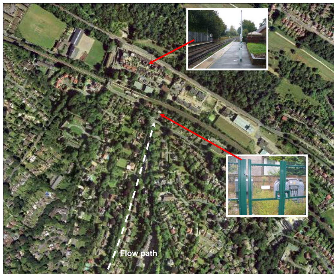
Figure 3-13 Pluvial flowpaths and receptors at risk on Kenley Lane, Kenley
